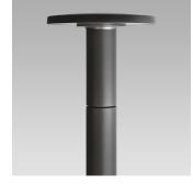
latest technologies for smart lighting and energy efficiency: MIKO Grande is the pole top luminaire for urban lightingwhich combines elegance and innovation with the highest quality of light, without producing light pollution. Die-cast aluminium body (EN 47100). Double layer polyester powder paint resistant to corrosion and salt spray fog. Silicone rubber gaskets. AISI 316 stainless steel external screws. Wiring on removable
