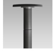
urban lightingwhich combines elegance and innovation with the highest quality of light, without producing light pollution. Die-cast aluminium body (EN 47100). Double layer polyester powder paint resistant to corrosion and salt spray fog. Silicone rubber gaskets. AISI 316 stainless steel external screws. Wiring on removable galvanized steel tray. Driver protected against voltage surges. High quality LED sources characterized
